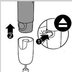
**9** Press the release button to remove the motor unit from the whisk coupling unit.
