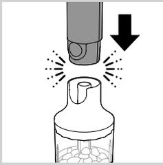
**4** Attach the motor unit onto the chopper lid (“click”).
