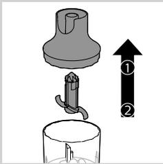
**9** Carefully remove the chopper lid and the blade unit (fig. 18).
