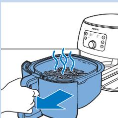
**12** Open the drawer by pulling the handle and check if the ingredients are ready.
