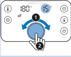
**9** To change the cooking time, turn the QuickControl dial to the desired setting.
