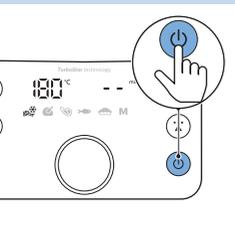
7 Press the Power On/Off (⏻) button to switch on the appliance.
