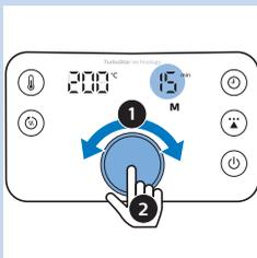
5 After the temperature is confirmed, the time indication “- -” starts blinking.
