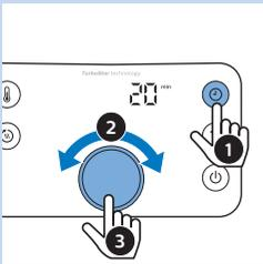
↳ The keep warm timer is set to 30 minutes. To change the keep warm time (1-30 min), press the timer button (🕒), turn the QuickControl dial and then push it to confirm. You cannot adjust the keep warm temperature.
