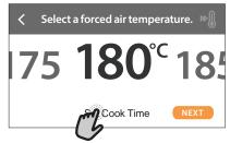
To cancel a set duration during cooking and so manage manually the end of cooking, tap the duration value and then select "STOP".
