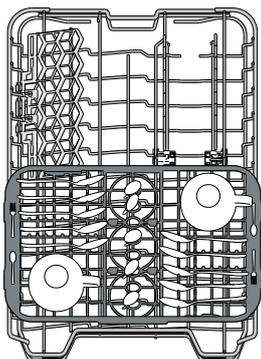
The upper rack is fitted with a sliding tray which can be used to hold small crockery and cutlery. For optimum washing performance, avoid positioning bulky crockery directly below the tray. The tray is removable.
