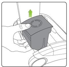
If the brush bar jams during use, the AirRAM K9 will stop and the LEDs will appear red. Before checking for a blockage, remove the battery.
