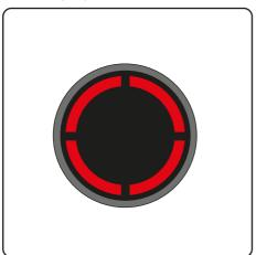
If the brush bar jams during use, the AirRAM K9 will stop and the LEDs will appear red. You will need to remove and clean the brush bar (see page 12).
