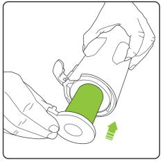
Slide the filter and inner shroud into the filter housing.
