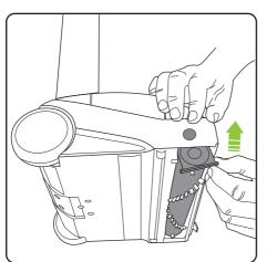
Re-insert the brush bar, starting by the end furthest away from the button. Then line up and push the brush bar into the AirRAM K9 until it clicks into place.
