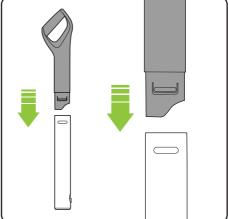
Fit the two components of the Upper Handle together in the orientation shown in the image above. They will only fit together one way. The components will click into place and will remain permanently fixed.
