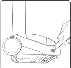
Rest the AirRAM K9 on its side and locate the brush bar button on the right hand side. Press the button inwards and then pull the brush bar out from the bottom of the AirRAM.
