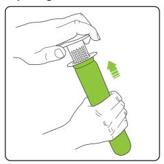
Slide the filter onto the inner shroud.
