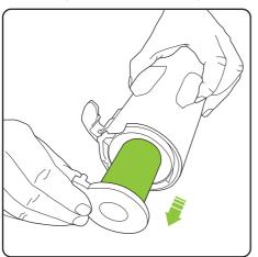
Slide the filter and inner shroud out of the filter housing.
