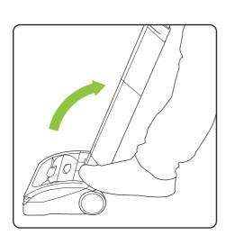
Press the power button with your foot to turn the AirRAM K9 on.
