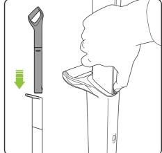
Insert the upper handle into the lower handle. You will need to press the button on the upper handle to fit it in.
