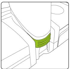
The green locking clip, when correctly fitted, will click and hold the lower handle in place. Should the handle assembly need to be removed the clip can be pulled out to unlock the lower handle.
