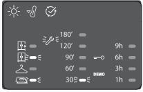
The presence of wrench symbol signals a malfunction. Carry out the operations described. Switch the dryer off and unplug it. Open the door immediately and pull landry out, to allow the heat to dissipate. Wait for about one hour. Reconnect the dryer to the power supply, load the laundry and restart the drying cycle.
