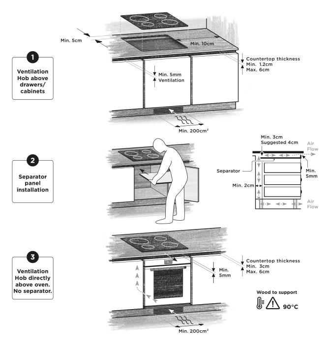
A separator/insulation panel needs to be installed between base of induction hob and storage space underneath hob respecting dimensions in diagram 1. No panel is to be installed if oven is installed under hob as in diagram 3.
