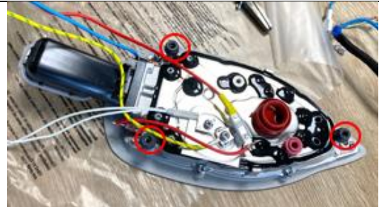
Assemble 3x Ryton Ring and dress all wires
