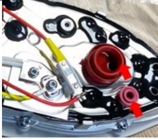
Assemble SOS SEAL 21 & DOSING SEAL 6 to SOLEPLATE ASSY 1
