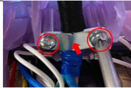
Assemble MAINSCORD 18, assemble Clamping Plate, assemble & fasten 2x Screw B
