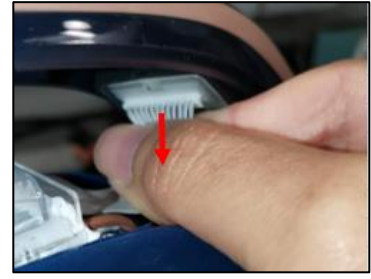
Make sure you hold all the cable and pull vertically to disassembly the Ribbon Cable
