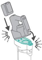
**1** To assemble the Vacuum & Mop set-up, insert the battery and attach the 3-in-1 handheld to the wet module ('click').
