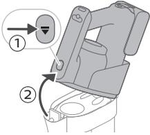
**2** Clean the inlet filter with a cloth or with the cleaning brush.
