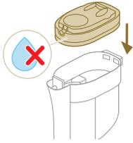
**⚠ Caution:** Make sure that the filter case including the foam filter are completely dry before you put them back into the dust bucket.
