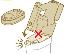
**⚠ Caution: Do not attach the 3-in-1 handheld to the dust bucket without the filter case being inserted in the dust bucket.**
