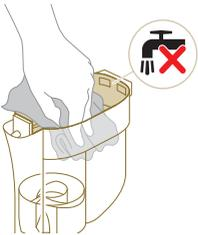
**i** Note: do not let the electronic connectors get wet. If the electronic connectors do get wet, please allow them to dry before using the device again. Always use the appliance with dry electronic connectors. This prevents the appliance from malfunctioning over time.
