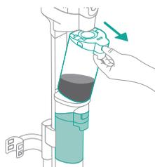
**14** Push the button to unlock the dirty water tank and remove it.
