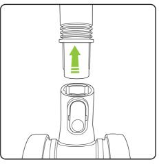
Gently pull the Power Brush from the product to remove. The battery should be removed when changing attachments.
