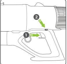
For continuous operation: press and hold the power button to switch on; press the lock button from either side.
