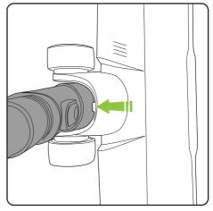
The handle will only remain upright if the interlocking notch and gap are engaged.
