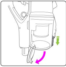
Hold the product over a rubbish bin and release the latch to empty the dirt. A gentle tap each time you empty the bin will help remove excess debris.
