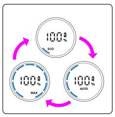
ECO – reduced power, longest run time Auto – adjusts to optimum power for the dust load conditions
