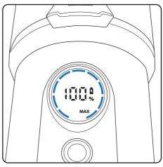
The display shows how much charge the battery has.
