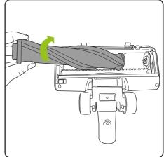
The brushbar rotates up and out, and can be removed for cleaning.
