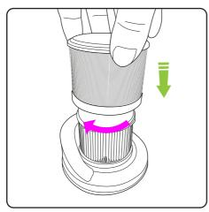
Push the metal shroud onto the filter and twist to lock in place.
