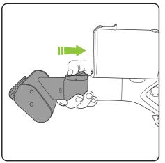
The small power brush is attached and removed in the same way as the power floor head.
