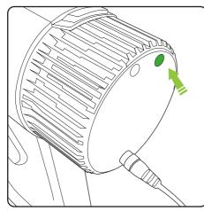
When charging the battery has a flashing green light. When fully charged the light will be continuous green.
