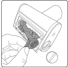
The brushbar can then be easily removed and cleaned.
