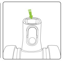
Remove the tube, floor head, dust bin, and any accessory tools and check through the openings for any blockages.
