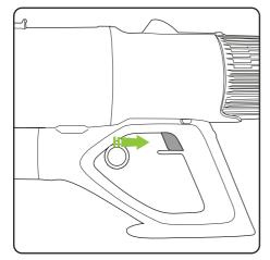
For short bursts of cleaning: press and hold the power button to switch on. Release the button to switch off.
