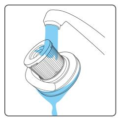
Tap the filter to remove any loose debris. The filter can be gently brushed but do not rub or scrub excessively.
