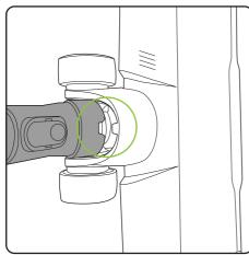
Engage the tube into the floor head when parking in the upright position.
