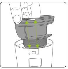
Return the filter assembly to the bin, lining up the tab on the filter with the recess in the bin.
