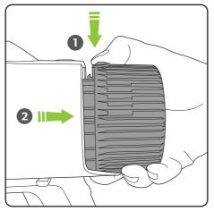
To remove the battery press the latch and pull the battery to remove from product.
