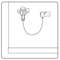
Consider position to be near a mains power socket if want to charge on the wall mount.
