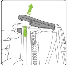
Slide the latch button inwards until the end plate disengages, then remove the end plate.
