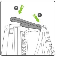
Push the latch into the slot by the brushbar then clip into place.
