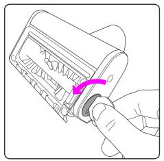
Using a coin or similar implement turn the end cap until it unlocks and remove it.
