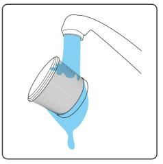
Wash both the filter and filter shroud under a tap with cold water.
