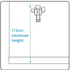
Install your wall mount at least 113cm from the floor. Screws and wall plugs have been included. Recommended drill size 6mm. Check the wall area is free of water pipes or electrical cables.
