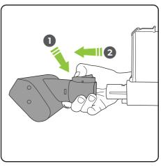
Like the power floor head, it can be attached directly to the AirFOX or to the extension tube.
