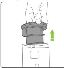
Remove the filter assembly from the bin.
