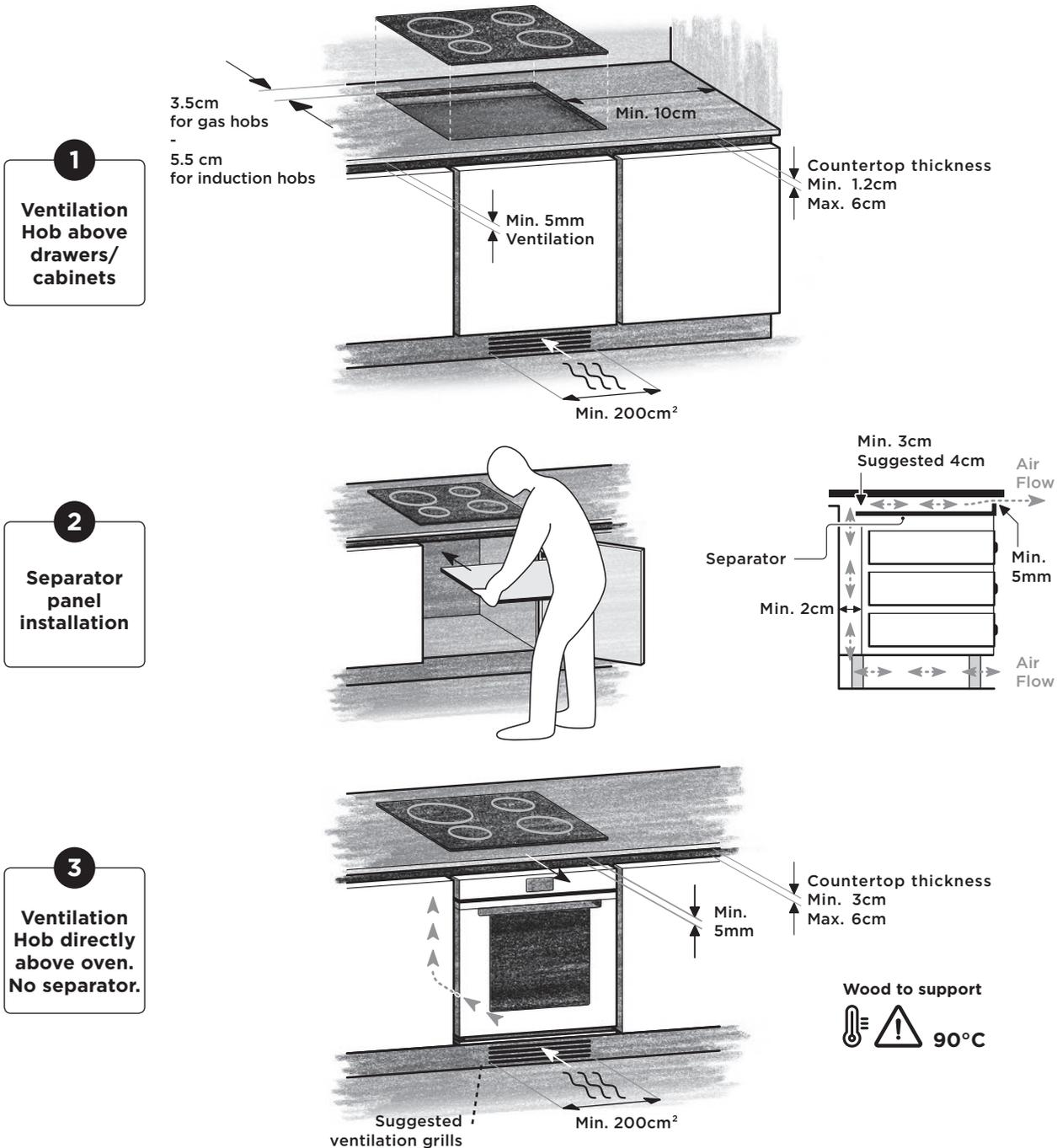
A separator/insulation panel needs to be installed between base of induction hob and storage space underneath hob respecting dimensions in diagram 1. No panel is to be installed if oven is installed under hob as in diagram 3.
